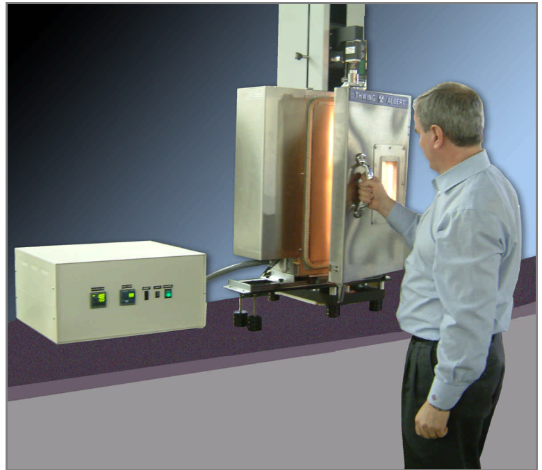
▲ The environmental chamber mounts on a single-column Vantage tester to measure the affect of elevated temperatures on material performance
