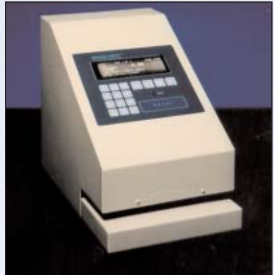
▲4340 Automatic Densometer & Smoothness Tester measures porosity and air-permeability of sheet-like materials
